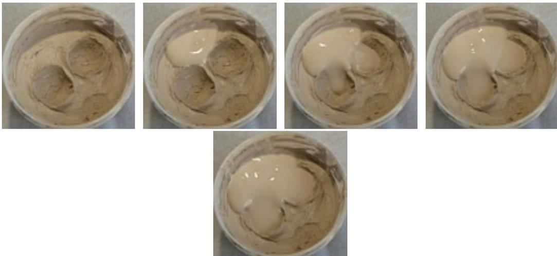
**Figure 5.** Endogenic lava flow creates a lava dome which has to rise enough to overflow the crater rims.
